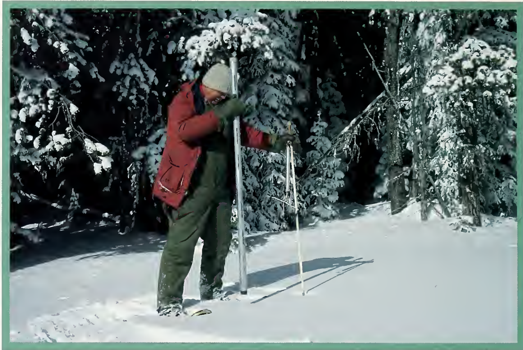
Snow depths and water equivalents are measured periodically at dispersed sites on Tenderfoot Creek Experimental Forest.
