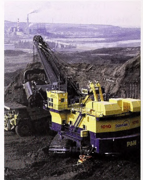
FIGURE 5.9.1-2 Large-Scale Commercial Oil Sands Surface Mining Activity North of Fort McMurray, Alberta, Canada (The shovel bucket holds approximately 100 tons of oil sands ore. An oil sands processing plant is visible in the background.) (Image courtesy of Suncor Energy, Inc.)
