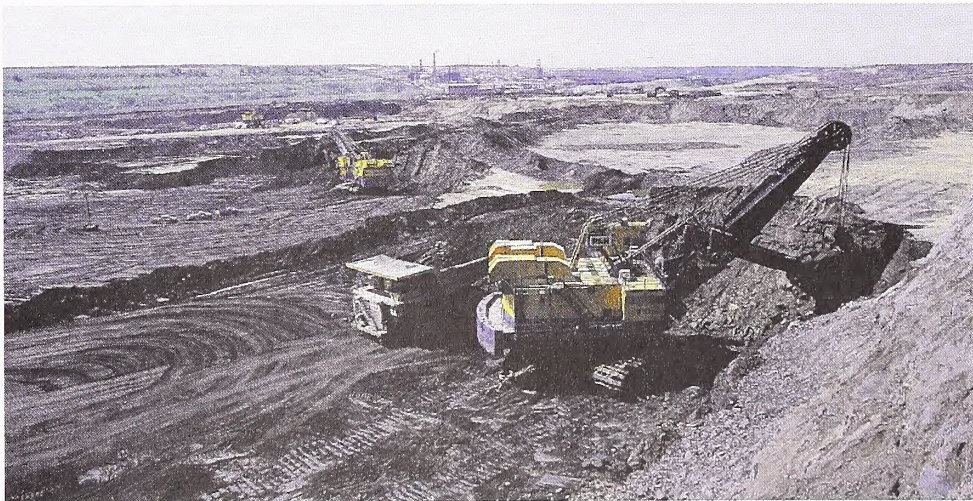
FIGURE 5.9.1-1 Large-Scale Commercial Oil Sands Surface Mining, North of Fort McMurray, Alberta, Canada (An oil sands processing plant is visible in the distant background.) (Image courtesy of Suncor Energy, Inc.)
