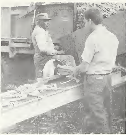
FIGURE 8.—Experimental equipment for mechanical stripping of celery stalks.
