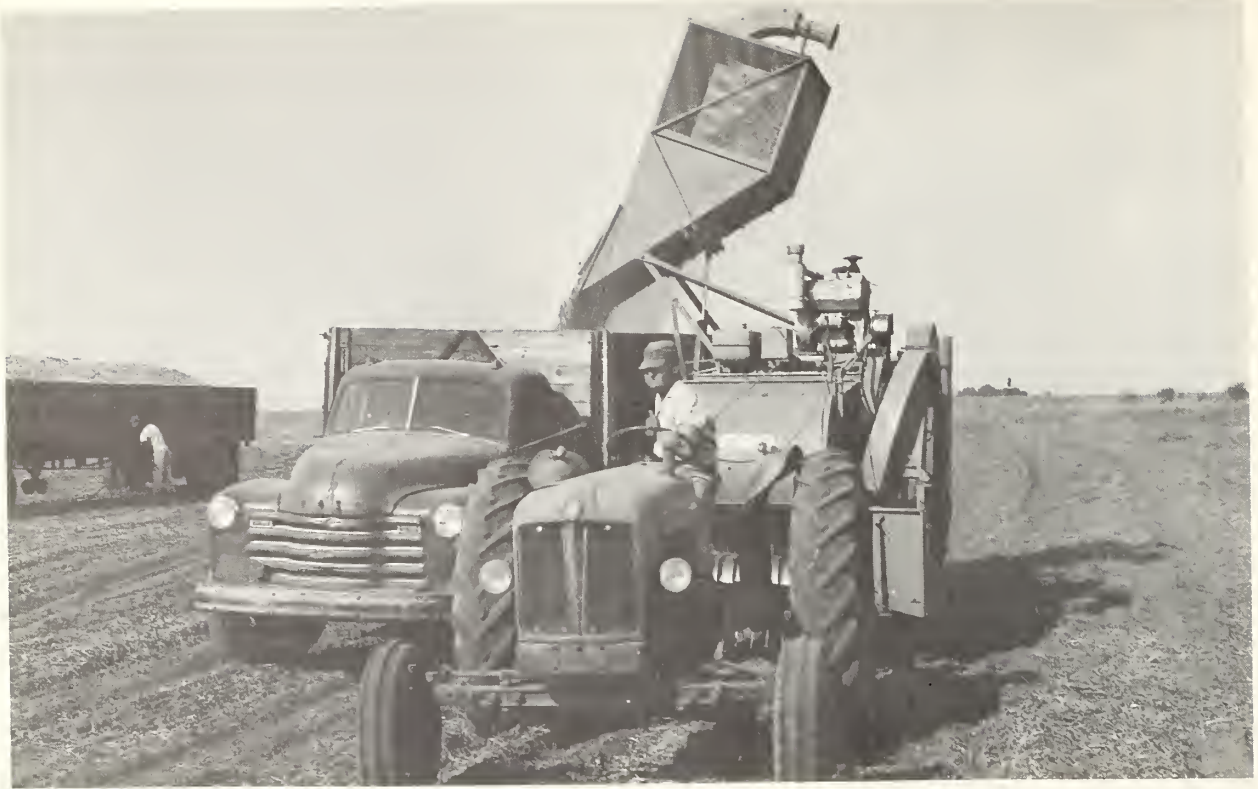
Bulk handling of peanuts. Combine dumps bulk peanuts into truck during harvest.
