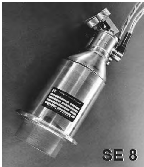
Saturn S IV B Stage Ullage & Apollo Command Module Reaction Control Engines (Source: Tim Harmon's presentation charts, Appendix F)
