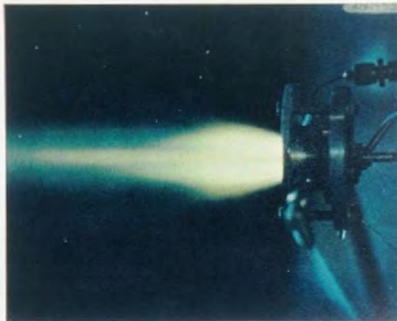
Plate 27. Concentric-Tube Injector of Plate 25 with 1.0-in.-long Chamber
