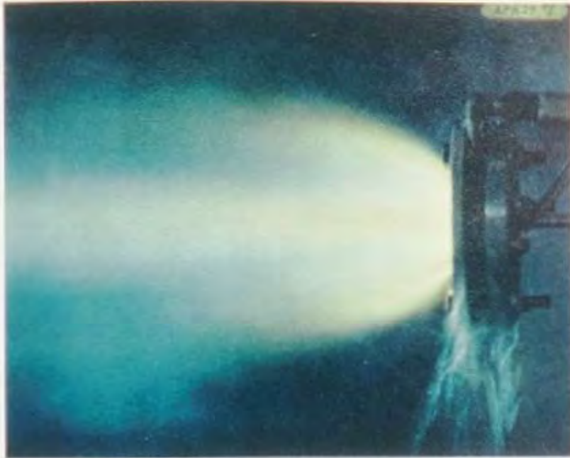
Plate 26. Concentric-Tube Injector of Plate 25 with 0.15-in.-long Chamber
