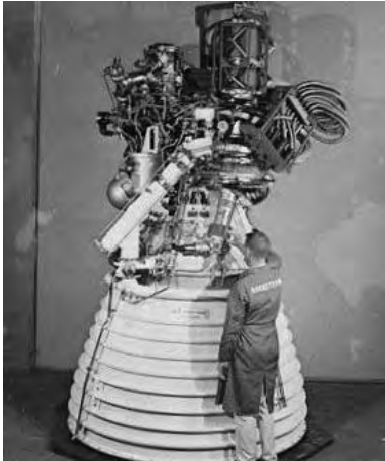
One of the J-2 engines that power the upper stages of Saturn V liquid hydrogen, on its way from the fuel turbopump, is used to cool the walls of the thrust chamber regeneratively. (Source: http://history.nasa.gov/SP-350 - Apollo Expeditions to the Moon", published 1975)
