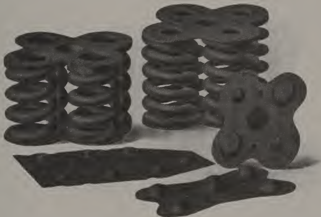
Fig. 16. Groups of Coil Springs held together by Plates at Top and Bottom
