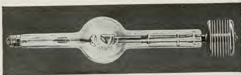
FIG. 2. SPECIAL SELF-RECTIFYING ROENTGEN RAY TUBE.
