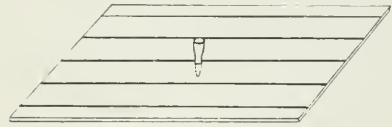
FIG. 4. RULED CELLULOID SHEET TO INDICATE EQUALITY OF MOTION OF TWO SHADOWS IN METHOD B.
