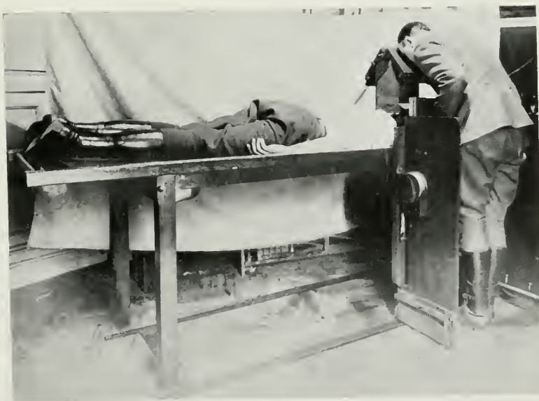
FIG. 3. STEREOFUOROSCOPE IN USE. TUBES AND SCREEN MAY BE SHIFTED IN THREE DIRECTIONS.
