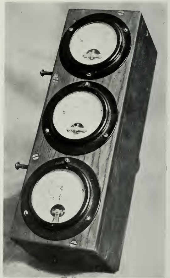
FIG. 8. METER PANEL DETACHED FROM THE MACHINE. SHOWING PRIMARY VOLTMETER, SECONDARY A-C. MILLIAMMETER, AND SECONDARY D-C. (LOAD BALANCING) MILLIAMMETER.
