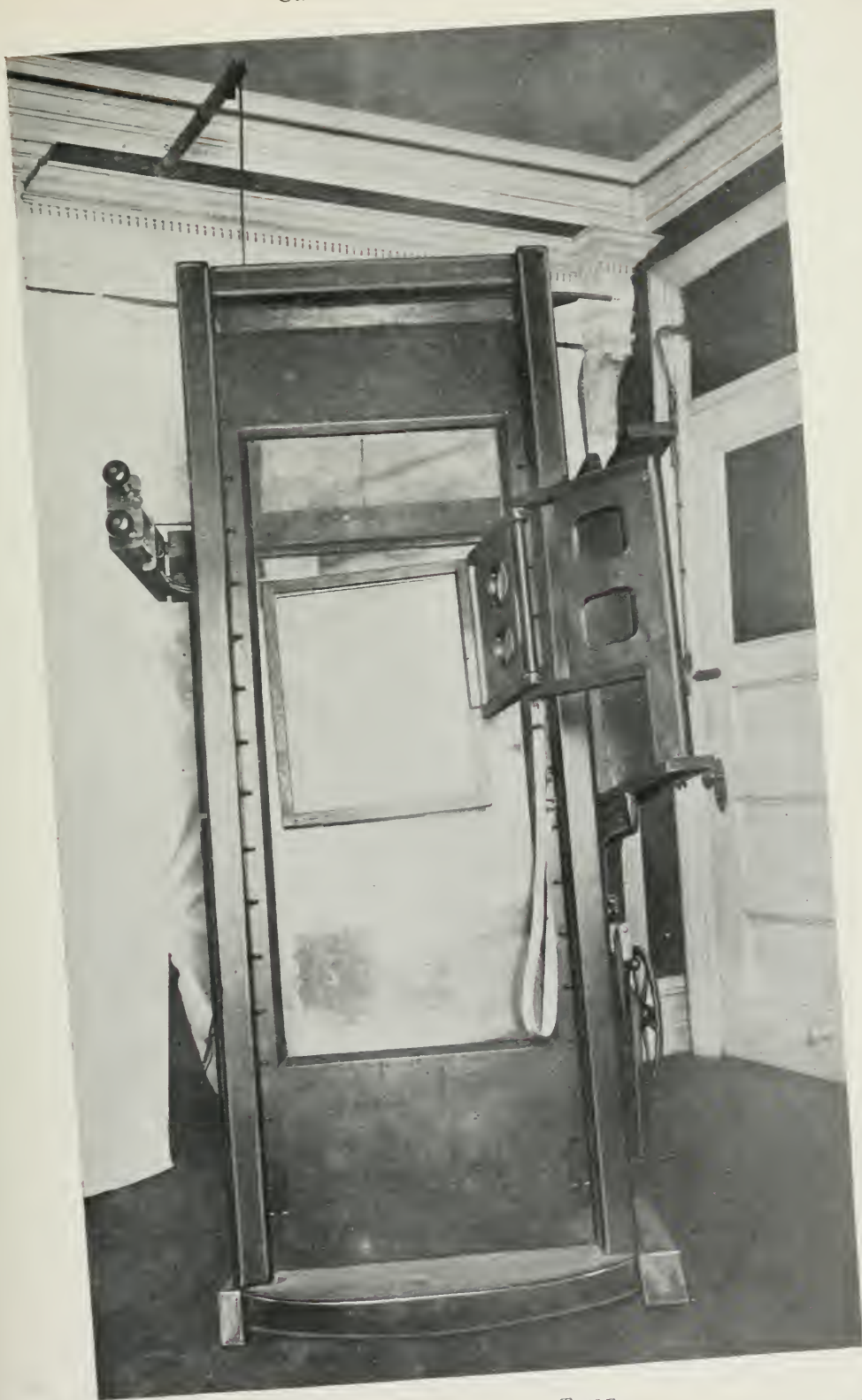
FIG. 1. CALDWELL TILT TABLE. with collimator back, the mechanism for the support of the fluorescent
