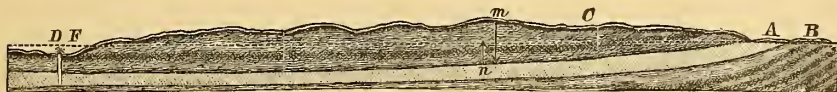
FIG. 66.—Section illustrating the aid afforded by a high water-surface between the fountain head and the well. (After T. C. Chamberlin; see Fifth Ann. Rept. U. S. Geol. Survey, fig. 15, p. 140.)
