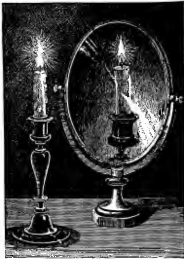
FIG. 19.—AN IMAGE FORMED BY A CONCAVE MIRROR.
