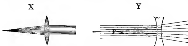
FIG. 36.—FOCUS OF PARALLEL RAYS OF CONVEX AND CONCAVE LENSES.
