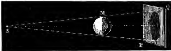
FIG. 7.—SHADOW OF SPHERE PRODUCED BY LUMINOUS POINT UMBRA ONLY PRODUCED.
