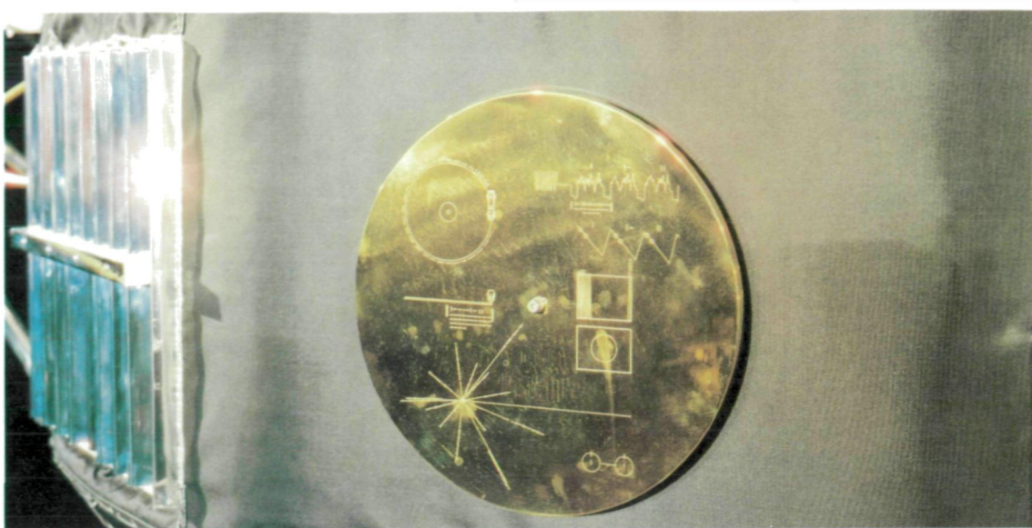
Each Voyager carries a message in the form of a 12-inch gold-plated phonograph record. The record, together with a cartridge and needle, is fastened to the side of the spacecraft in a gold-anodized aluminum case that also illustrates how the record is to be played. [P-19728]
