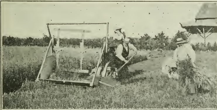
FIG. 10.—Early type of reaper developed about 1830. The grain was raked from the platform by hand. This machine evolved finally into the self-rake reaper still used in this country for harvesting flax and buckwheat.
