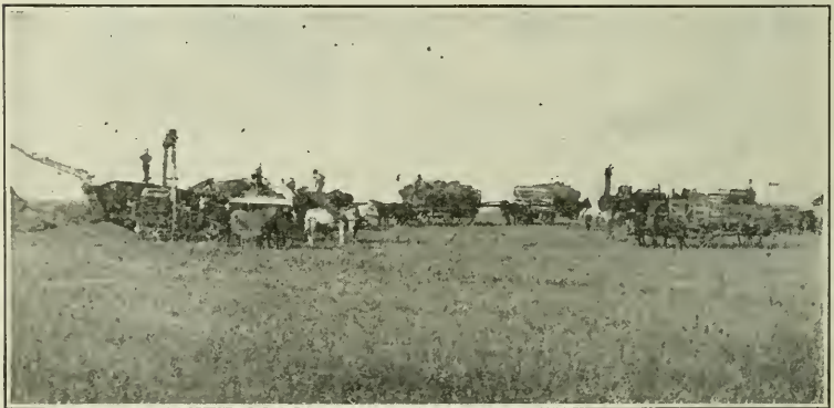
FIG. 16.—The modern grain separator, developed with the self-binder, thrashing wheat from the shock by steam power from a traction engine.
