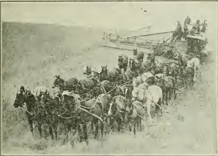
FIG. 17.—A large-sized combined harvester-thresher or "combine," drawn by 32 horses and cutting 30 to 40 acres daily. Smaller sizes are becoming popular and tractors often are used for power. These machines cut and thrash the grain at the same time. These and headers are used under dry-land conditions.
