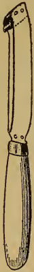
FIG. 38. Girdling knife, made of two thin steel blades with cleaner at a.
