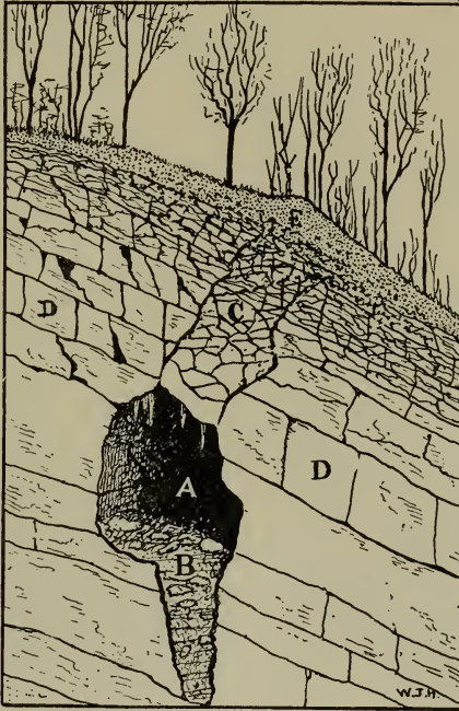
FIG. 1. Diagrammatic section of the cave before its walls were removed in the process of blasting and excavation. A. Open chamber. B. Space filled with earth and stones in which bones were found. C. Fissure closed with rocks. D. Limestone strata dipping to the south. E. Soil bearing forest growths.
