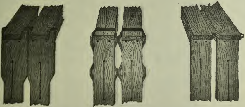
Fig. 6.—(a) Hoffman self-spacing frames.
