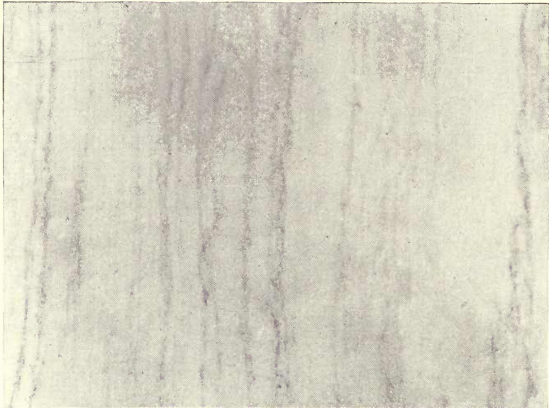
Fig. 169.—Polished slab of listavena marble, West Rutland, Vermont. Photo. by C. H. Richardson.
