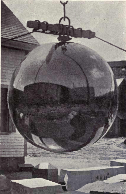
Fig. 46.—Ball of polished Quincy granite from the Wigwam quarries, Quincy, Massachusetts. Diameter 76 inches. Weight 22,010 pounds. By courtesy of the U. S. Geological Survey.
