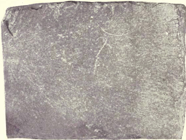
Fig. 248.—Slab of clay slate, Northfield, Vermont, showing perfect cleavage. Photo. by C. H. Richardson.
