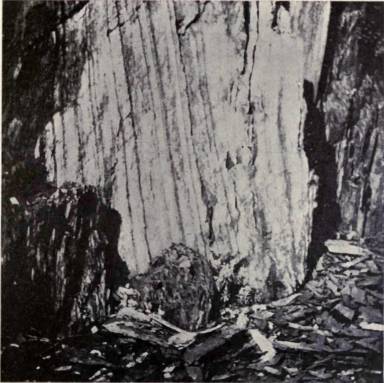
Fig. 249.—Sabin slate quarry, Northfield, Vermont, showing the difference between the cleavage and bedding planes. Photo. by C. H. Richardson.
