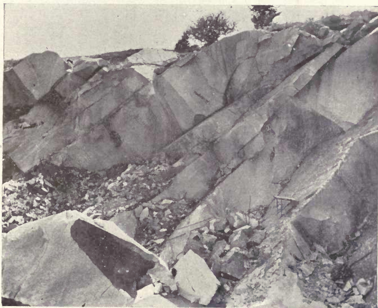
Fig. 80.—The Patch Company granite quarry, Calais, Vermont, showing thickness and steep dip of sheets. Photo. by C. H. Richardson.
