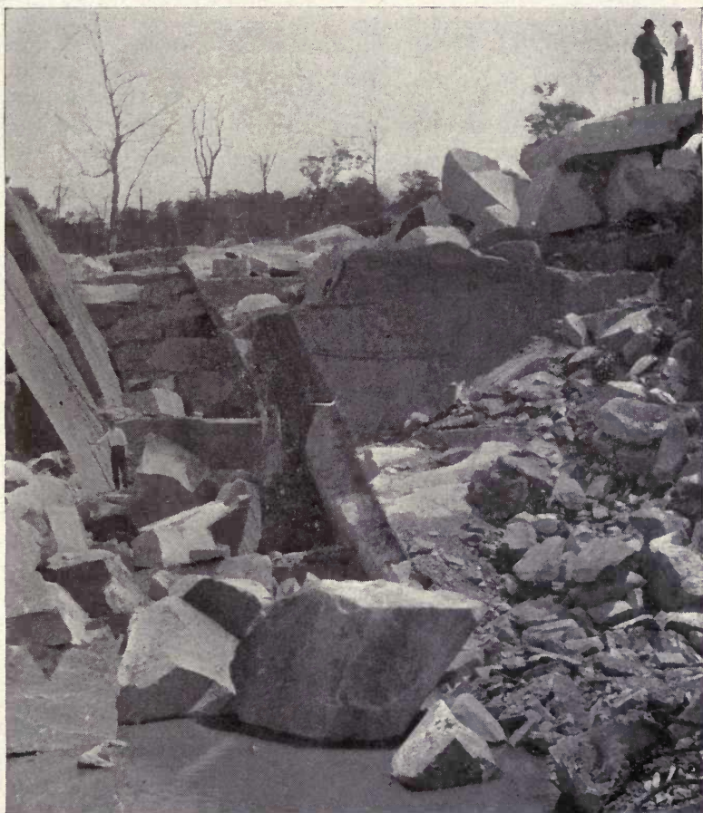
Fig. 87.—Imperial blue granite quarry, Buck Lake district, Woodbury, Vermont, showing head seams. Photo. by C. H. Richardson.
