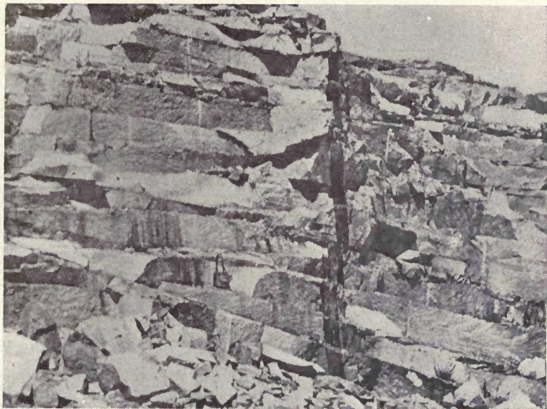
Fig. 35.—Allen quarry, west side of Somes Sound, Mount Desert, Maine, showing lenticular sheets crossed by a vertical diabase dike, faulted on the fourth sheet from the bottom of the quarry. By courtesy of the U. S. Geological Survey.
