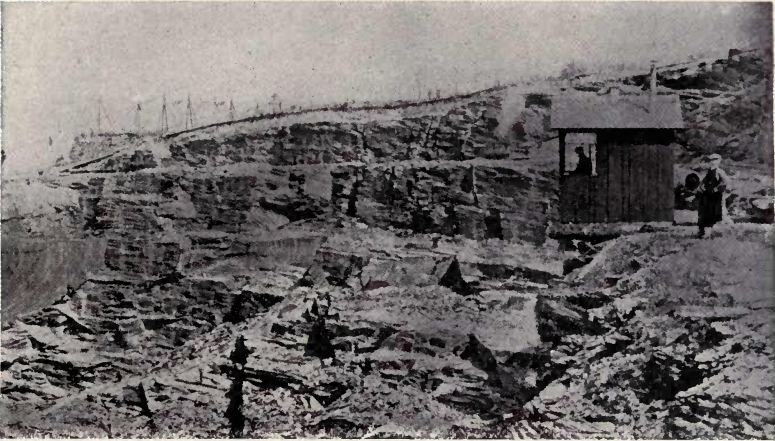
Fig. 243.—Old Bangor slate quarry, Bangor, Pennsylvania, showing the close overturned syncline crossed by almost horizontal cleavage. By courtesy of J. S. Moyer.
