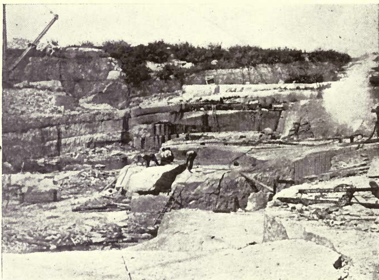
Fig. 40.—Sands quarry, Vinalhaven, Maine, showing the curvature of the sheets, the intersecting joint face and the north 10^{\circ} east channelling along the cut-off. By courtesy of the U. S. Geological Survey.
