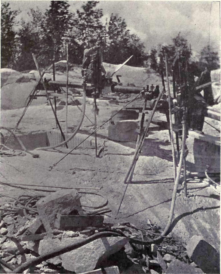
Fig. 106.—Channelling machine at work on Wetmore and Morse quarry, Barre, Vermont. Photo. by C. H. Richardson.
