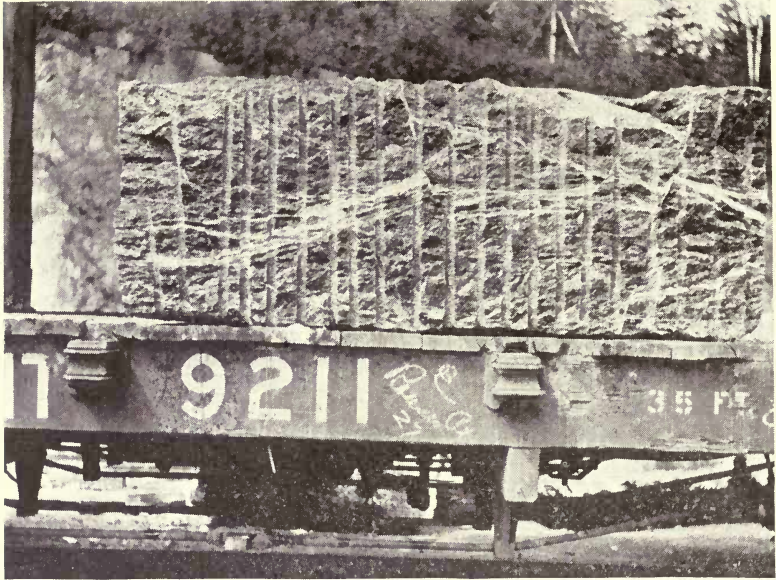
Fig. 256.—Rough block of verd antique marble, Roxbury, Vermont, showing work of channelling machine. Photo. by C. H. Richardson.
