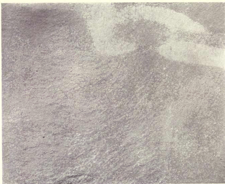
Fig. 9.—Slab of red slate from Granville, New York, showing a white vein-like band formed by the leaching out of the pigment in the slate. Photo. by C. H. Richardson.
