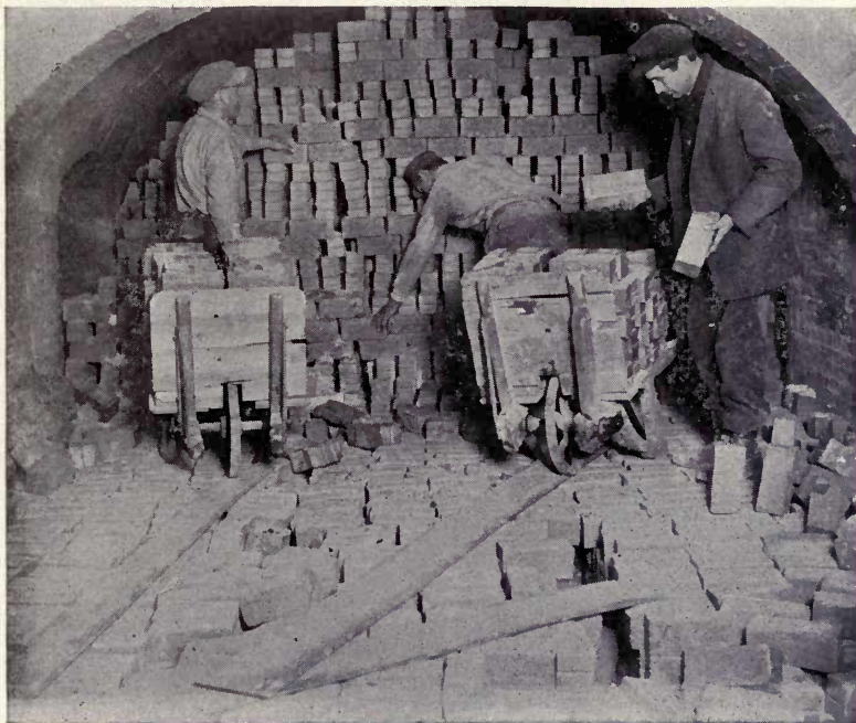
Fig. 290.—A scene showing how a section of the continuous kiln is being emptied of brick ready for market. By courtesy of the National Paving Brick Manufacturers Association.
