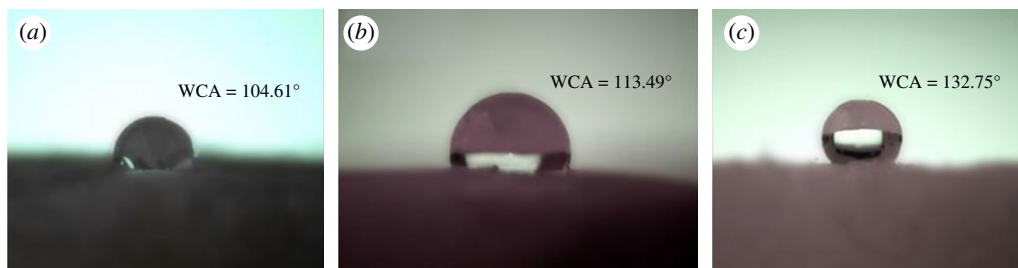
Figure 6. Water contact angle of the (a) HPSA-0, (b) HPSA-1 and (c) HPSA-2.
