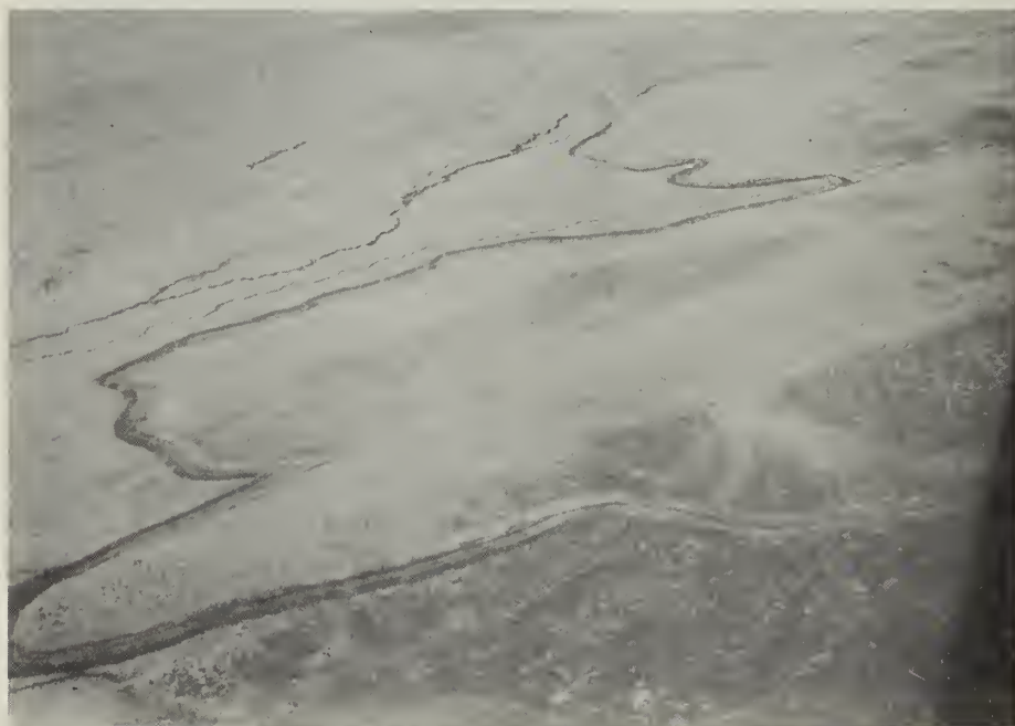
Photograph 21. -View of a diversion ditch to pick up runoff waters and carry it to a dry lake bed. The dry lake is just to the right of the area shown.
