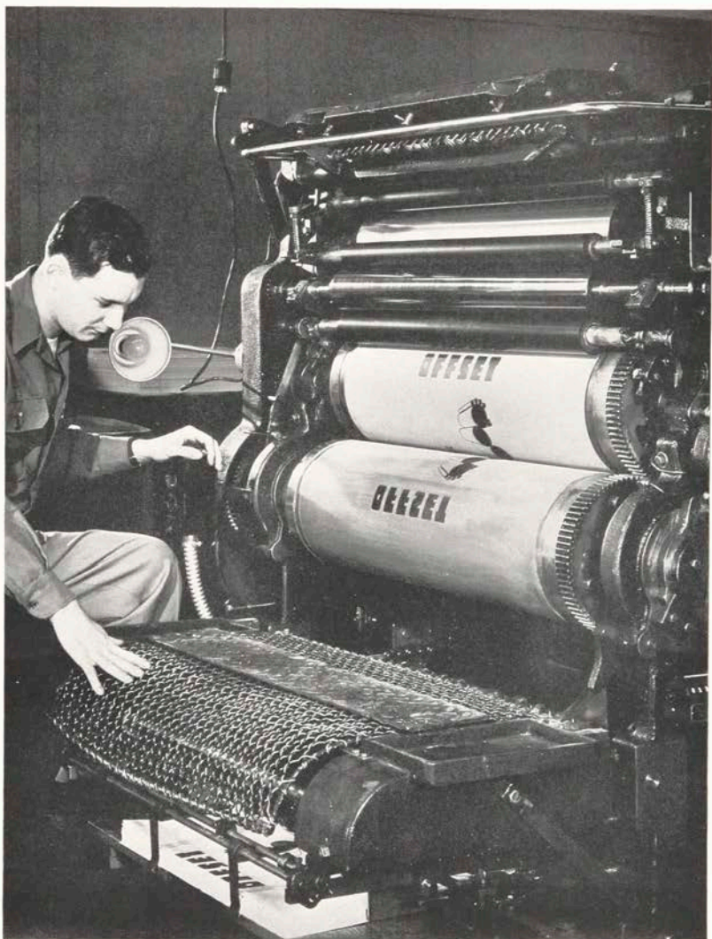
The four-color frontispiece and the two-color division pages of the 1949 Techmila were lithographed on this ATF Big Chief, 22 by 29, offset press.
