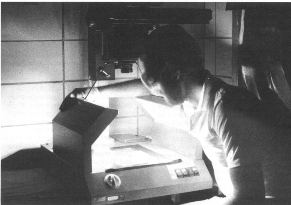
An ultraviolet system detects plasmid DNA molecules that control characteristics such as butter aroma or acid production in dairy product fermentation.
