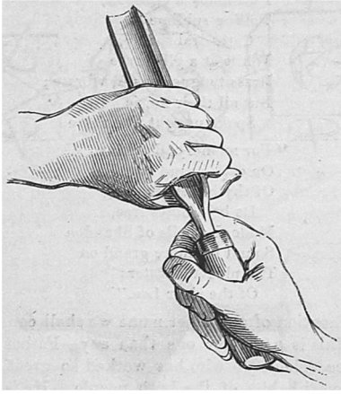
FIG. 1.—METHOD OF HOLDING THE GOUGE.
