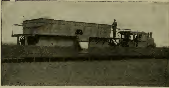
Showing Feed Distributing Car, Capacity 50,000 Lbs. Per Hour.
