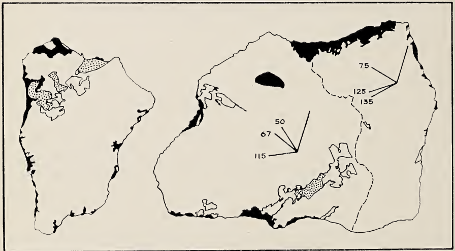
FIGURE 4. Tracings from photographs of etched surfaces shown in Figure 3—black: oxidation, white enclosed areas: schreibersite, dotted: troilite. Dashed line indicates composition surface between two parts of twin. Radiant diagrams show angles between kamacite bands limited to one part of twin and those shared in common (longer line).
