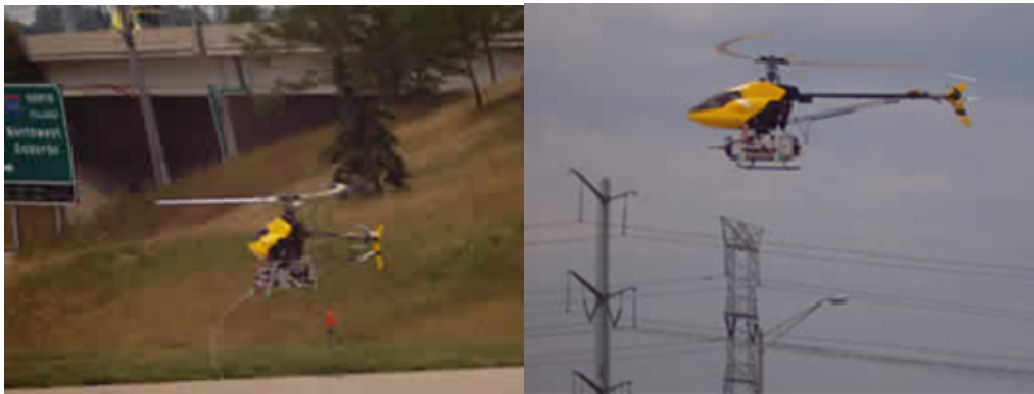
Figure 19. Autonomous Highly Maneuverable Miniature Helicopter (AHMMH-1) used in ONR-STRR program 68
