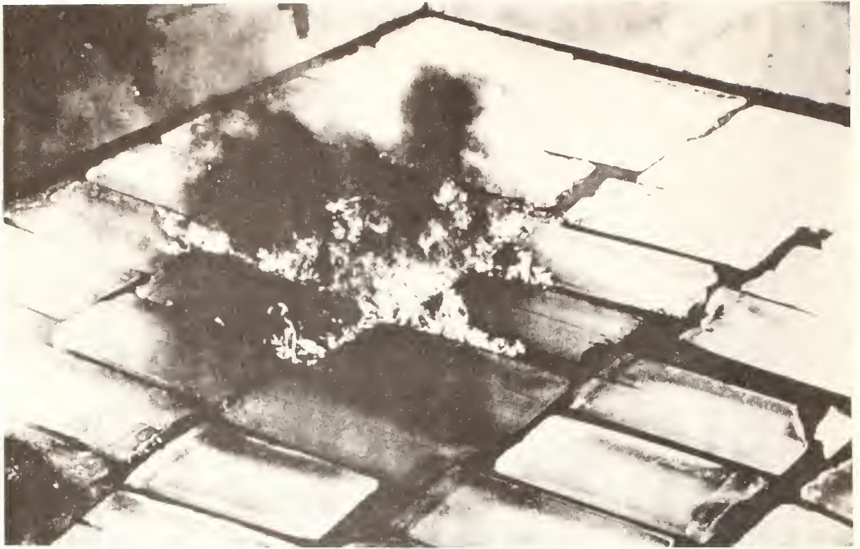
Figure 12 Demonstrating the burnability of an emulsion of 92% Prudhoe Bay crude oil and 8% bay water in tests at OHMSETT [3]
