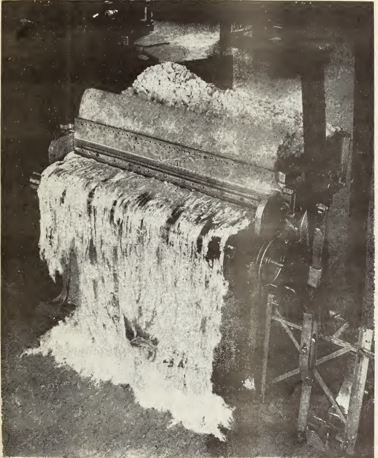
Figure 5.- Slow-speed lint doffer for roller gins.
