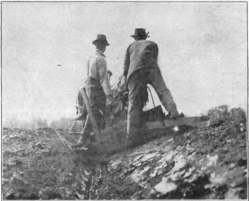
FIG. 33.—A steel ditcher and terracer. Four horses are generally used with this implement in terracing work.
