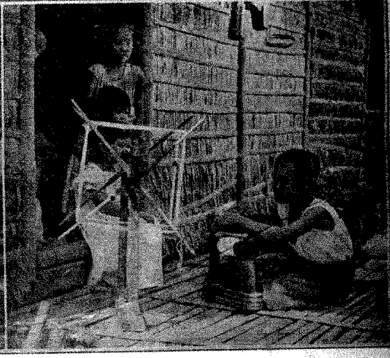
Winding up the Fiber on Spools for Use in Making Fine Fabrics.
