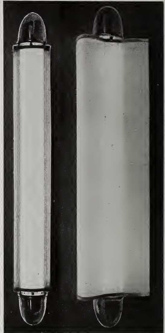
The left hand shield above is made of two shapes of extruded plastic, the center of greater diffusion in a ribbed design, while the edges are extruded tubes of clear colored plastic. This gives a higher brightness color accent to the edges. The proportions of the unit as well as the form are changed by applying other extruded plastic shapes (right hand). The center is a flat ribbed section that gives a band of higher brightness in contrast to the more diffusing and softer glow from formed side sections.
