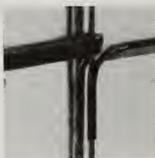
How the tool is used: Figure 1 (left) shows a Wagner frame bar out of line; Figure 2 (left-hand below) adjusting bar with tool; and Figure 3 using tool to measure angle. The tool must fit the face of the horizontal bar flush.
