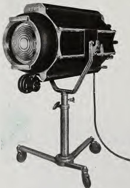
Remarkable Klieglight with 3000-watt incandescent light source; Fresnel lens and auxiliary spread lens; forced-draft air-circulating system; ellipsoidal Alzak reflector; and inbuilt iris and curtain shutters.
