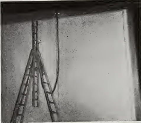
Setting up for mechanical screen resurfacing (above). The track starts at top and carries the spray gun (see detail view below) across the screen in downward steps.
