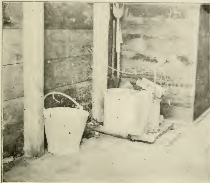
Model device for dumping cyanide into acid from exterior of house. Planned and in use by Mr. Wright at Windsor.
