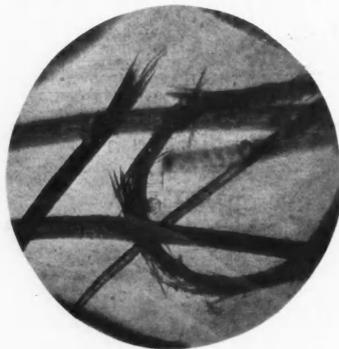
FIG. 3. Fiber attacked by bacteria showing brush-like ends, and splintered appearance. (About 500 diameters.)
