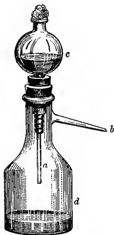
FIG. 15.—Kitasato's filter: a , porcelain bougie; b , attachment for suction-pump; c , reservoir; d , sterile receiver.
