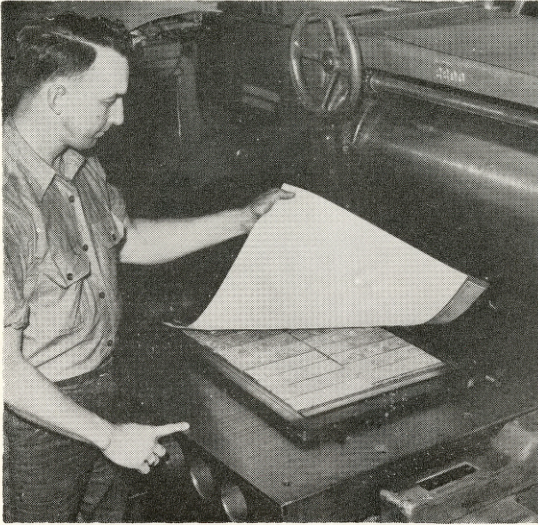
Stereotyper lays matrix paper on page form to be run through mat roller under pressure of 500 pounds per square inch.
