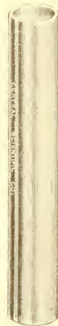
FIG. 6.—Twelve-inch tube with solid bottom, for use in determining volume-weight and pore space.
