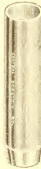
FIG. 5.—Soil sampling tube for taking a sample of surface soil in an undisturbed condition—useful in determining the volume weight of soil in its field condition
