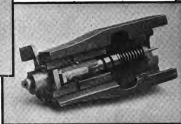
THE INNER SIDE OF THE BREECH BLOCK COVER WITH FIRING-PIN COCKED.
