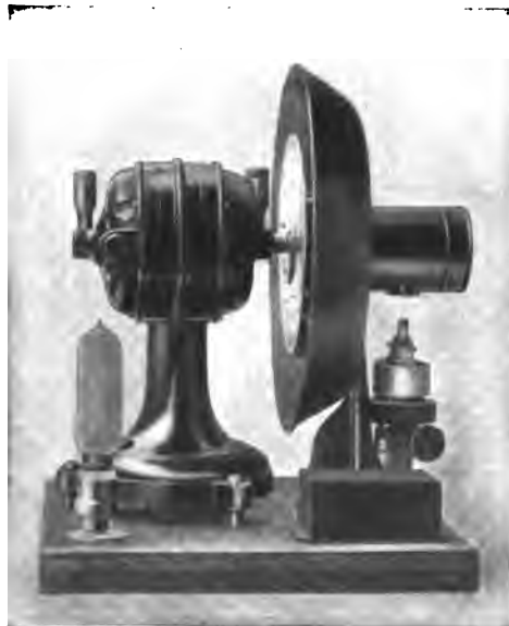
OZONE FAN CONSTRUCTED BY DR. FISCHER. This fan concentrates the ozone in the atmosphere.
