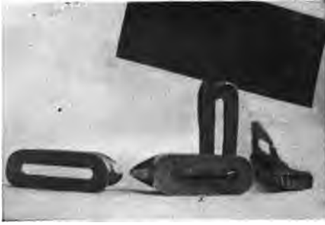
CASTINGS WORN BY FRICTION OF PAPER.
