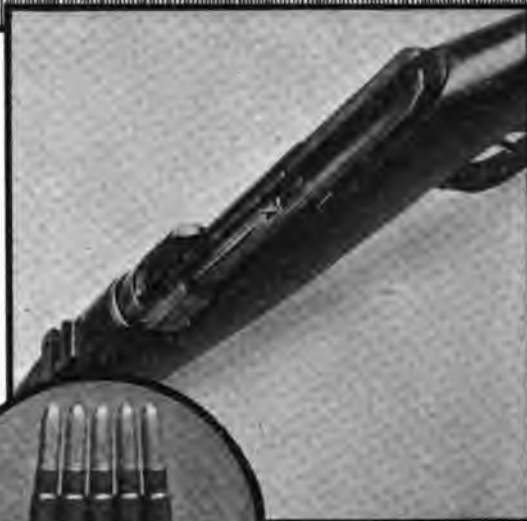
VIEW OF BREECH MECHANISM WITH BLOCK COVER REMOVED, AND ALSO BOLT-LOCK PIECE.
