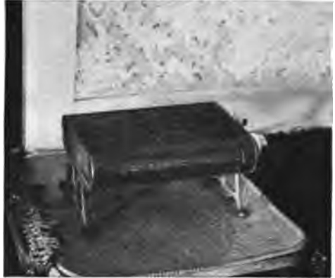
ELECTRIC HEATER MADE AT HOME BY A BOY.
