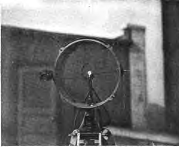
THE WHITE-HOT MAGNESIA BUTTON. Parabolic reflector not yet in place.
