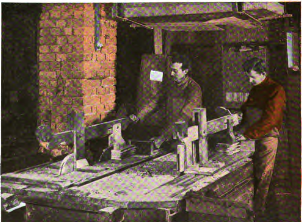
PROTECTIVE DEVICE ON CIRCULAR WOOD SAW TO PUSH FORWARD SMALL BOARDS.
