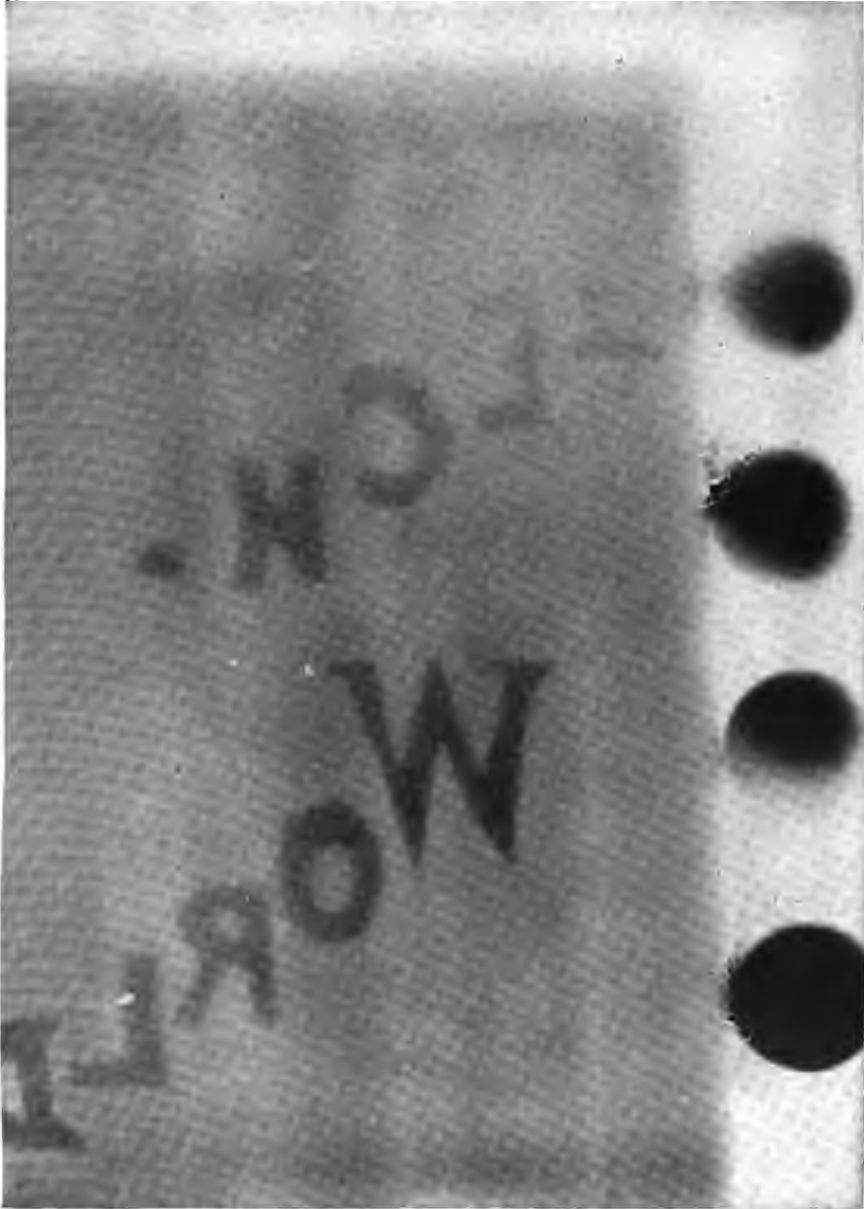
PHOTOGRAPH TAKEN THROUGH A BOARD WITH THO-RAD-X.
