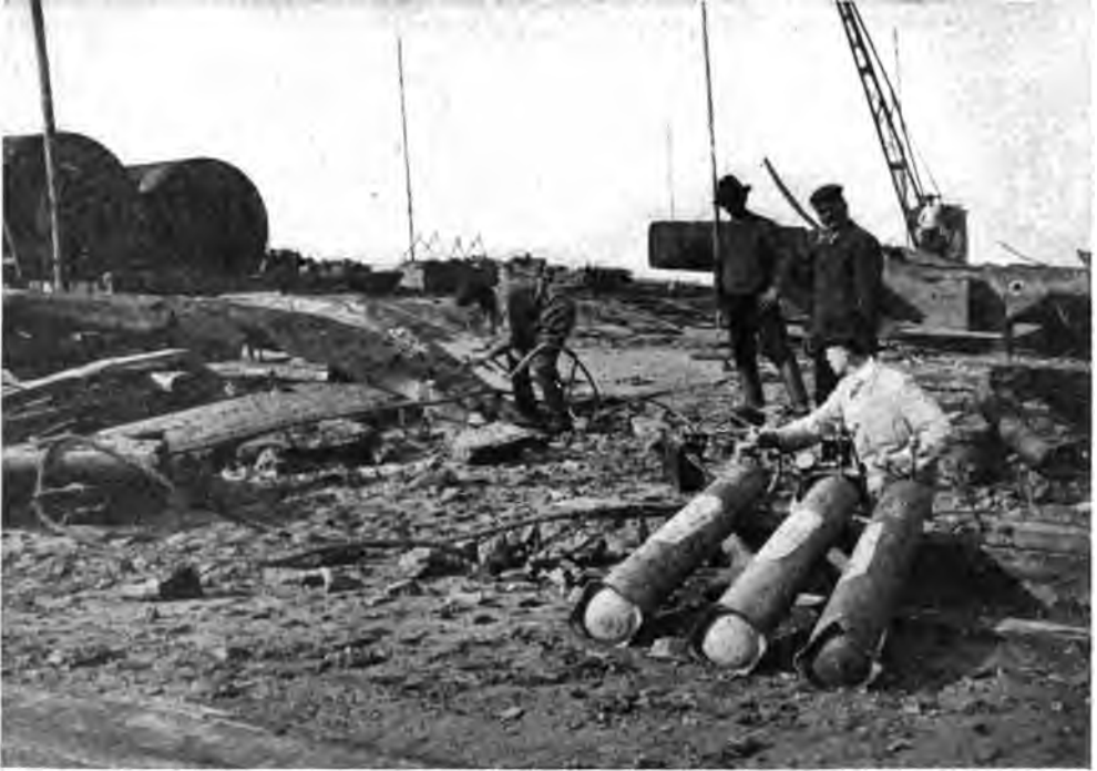
THE OXY-HYDROGEN BLOW-PIPE DEMONSTRATING ITS ABILITY TO CUT AN ARMOR PLATE SEVEN INCHES THICK.
