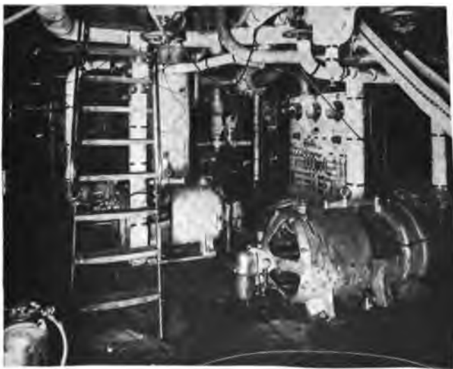
HORIZONTAL CURTIS STEAM TURBINE SET IN ENGINE ROOM OF THE Hendrick Hudson . ONE OF THE TWO LARGEST RIVER STEAMERS FLYING BETWEEN NEW YORK CITY AND ALBANY.
