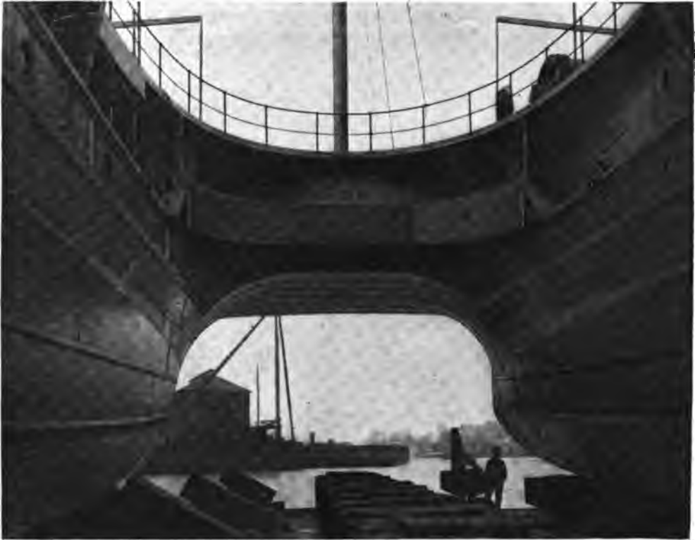
SMALL VESSELS MAY PASS UNDERNEATH. Note the peculiar double-ship construction.
