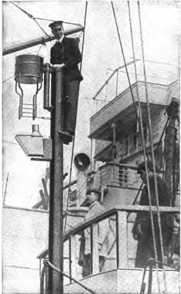
HOW THE SHIP'S COMPASS WAS ARRANGED SO AS TO BE FREE FROM ALL INCIDENTAL MAGNETIC INFLUENCES.
