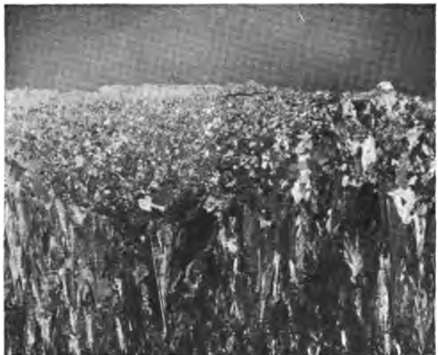
MICROPHOTOGRAPH OF DEPOSITED COPPER, SHOWING CRYSTALLINE STRUCTURE.
