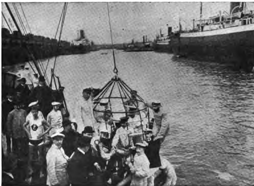
LIFE-SAVING CAGE. SHOWING MANNER IN WHICH IT IS CONTROLLED BY CORD AND PULLEYS.
