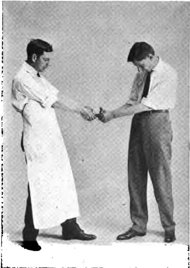
TRYING TO PULL PLUG AND RING GAUGES APART AFTER EXPANDED FROM HEAT OF HAND.
