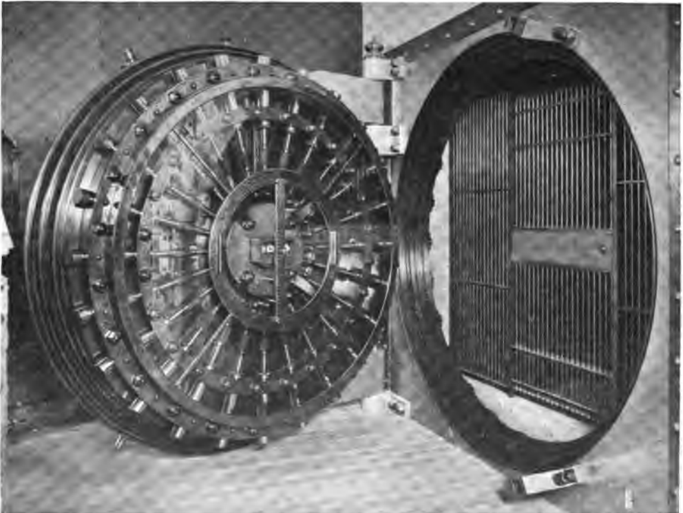
DOOR OF VAULT, SHOWING HAND-FINISHING ON PARTS OF LOCK MECHANISM.
