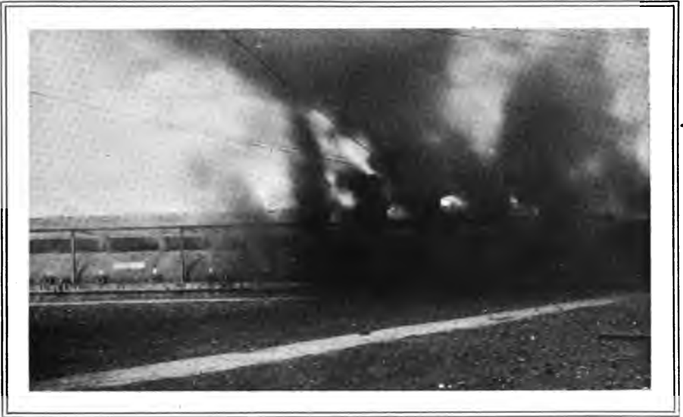
FIFTEEN SECONDS AFTER AN EXPLOSION OF COAL DUST IN THE EXPLOSIVES GALLERY.
