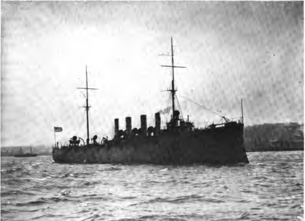
THE BIRMINGHAM . EQUIPPED WITH RECIPROCATING ENGINES. She has been surpassed in speed by the turbine-propelled steamers, Chester and Salem .
