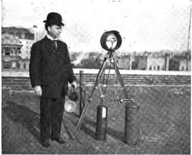
THE SENDING AND RECEIVING TRIPLE MIRROR OUTFIT. Triple mirror in operator's hand.
