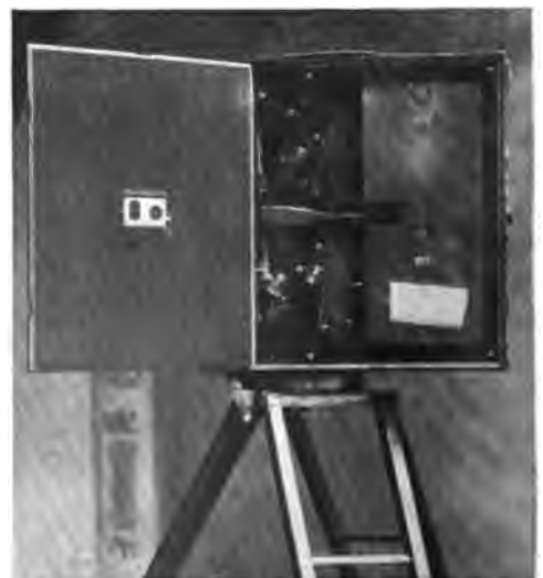
INTERIOR OF ONE SIDE OF CAMERA. The operating mechanism with reference to the sensitized film and the color filter band.
