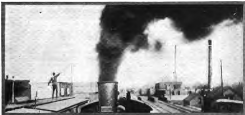
SAME ENGINE USING RAW COAL.
