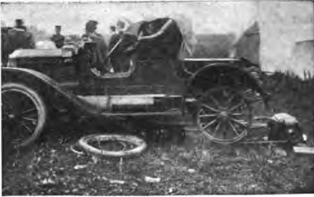
RUNNING AN AUTOMOBILE TO GENERATE POWER FOR ELECTRIC LIGHTS.
