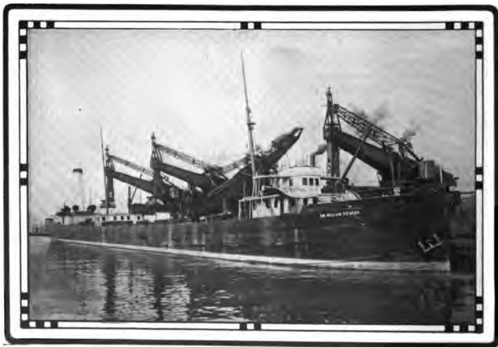
THE LAKE TRAFFIC IN IRON ORE. Automatic machinery unloading a vessel.
