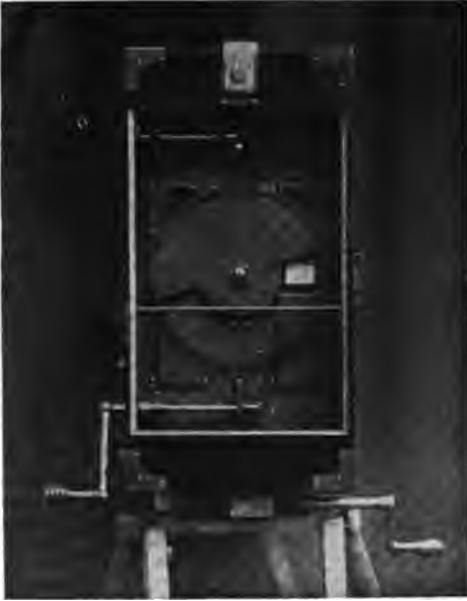
A. FRONT OF CAMERA WITH LENSES REMOVED, SHOWING SHUTTER ARRANGEMENT. Lens with the blue filter is exposed, the other lens is shut.
