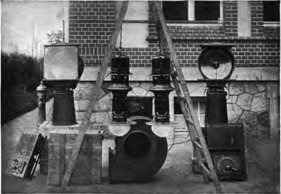
THE APPARATUS FOR LURING AND DESTROYING THE BUTTERFLY PEST. The principal parts are two electric search-lights, with dispersing mirror, suction fan and collection box.
