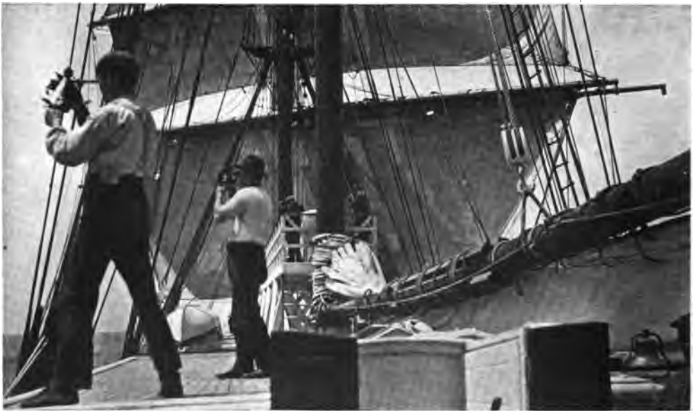
"TAKING SIGHTS" ON THE GALILEE , ON HER CRUISE IN THE PACIFIC OCEAN. Inasmuch as iron was used in her construction, the magnetic survey did not find this vessel quite adequate for their purposes.
