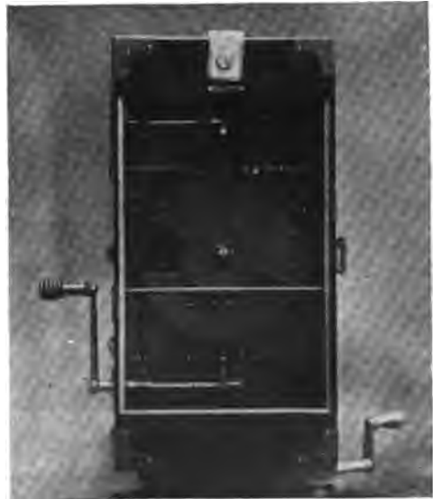
B. SHOWING SECOND LENS EXPOSED WITH BLUE FILTER. A and B show alternating motion of shutter and exposures.
