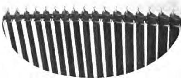
BLADING OF PARSONS TURBINE. SHOWING SHROUDING AND THINNING OF BLADE TIPS.
