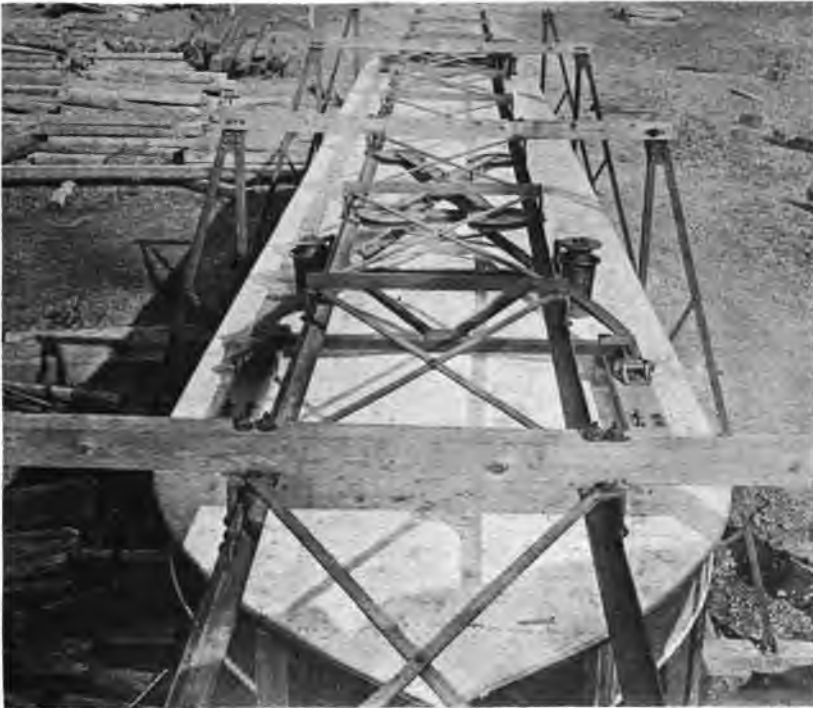
LOOKING DOWN ON TOP OF THE MONORAIL CAR. This view shows the overhead guide-rails to advantage.
