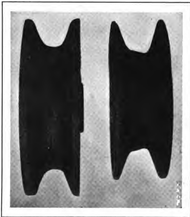
TWO TROLLEY WHEELS OF DIFFERENT SIZES. The larger was treated by the Lamon method and shows no sign of wear after traveling over 8,000 miles. The smaller wheel ran but 1,200 miles, wearing down as the photograph proves.
