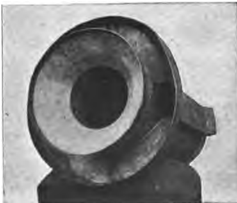
LOOKING DOWN UPON THE TOP OF THE NEW SPARK-PROOF LOCOMOTIVE SMOKESTACK.
