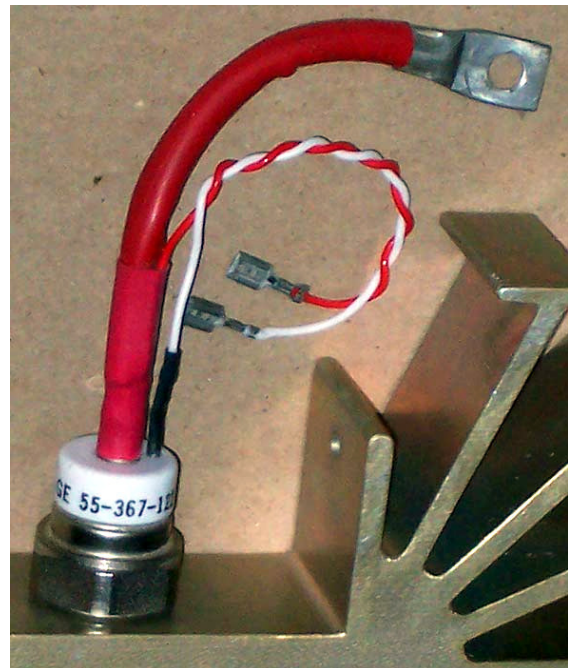
An SCR rated about 100 amperes, 1200 volts mounted on a heat sink - the two small wires are the gate trigger leads
