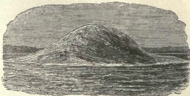
FIG. 113.— Explosion of 432 lbs. of Gun-Cotton in 37 feet of Water.
