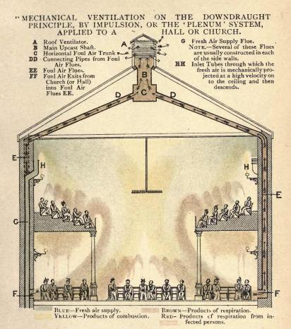
"In halls arranged with galleries, the difficulty of so arranging downward currents that, on the one hand, the air rendered impure in the galleries shall not contaminate that which is descending to supply the main floor below, and, on the other hand, the supply for the floor shall not be drawn aside to the galleries, is so great that it is almost an impossibility to effect it."— Extract from Government Report to Congress on the failure of mechanical ventilation at the Capitol, Washington, U.S.A.
