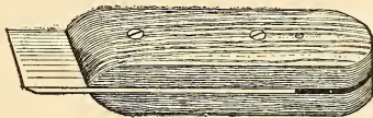
FIG. 106.—Knife for freezing microtome, made from the blade of a carpenter's plane.
