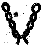
A CAT'S-PAW, FOR SETTING UP SHROUDS, ETC.
