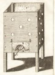
A The mouth of the Furnace B The Cover C An iron Peel D The Cnamel to be melted E The Grates T The inner part of the Furnace
