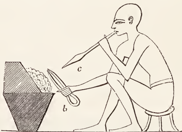
405. Blowpipe, and small fireplace with cheeks to confine and reflect the heat. Thebes.
