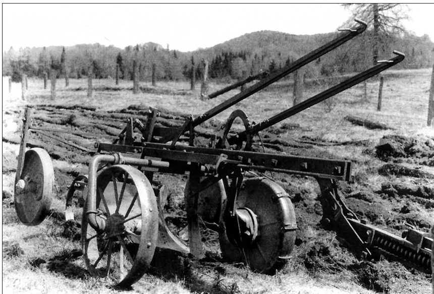
Figure 2.128. Preparing for planting in spring 1934 with the Heiberg Reforestation Plow, looking southeast across Plot 37 east of Creek Road on the Tompkins Farm. This plot was known as the “Heiberg Plow Plantation.” (Photograph 48-22:4000 [12], Franklin D. Roosevelt Library.)
