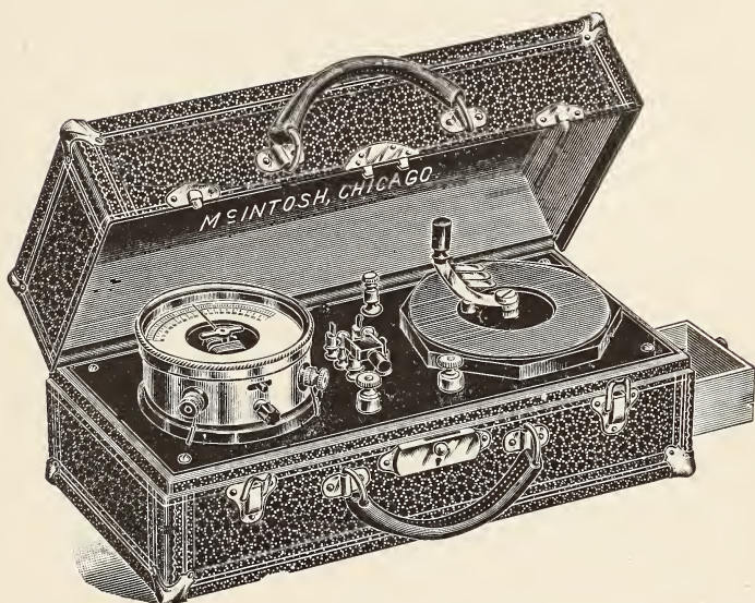
Portable Battery Indicated in Dr. Granger's Paper.
