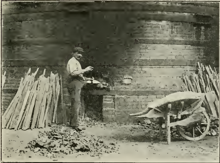
Putting salt on fires to form the salt glaze on wares, Swansea, Ont.
