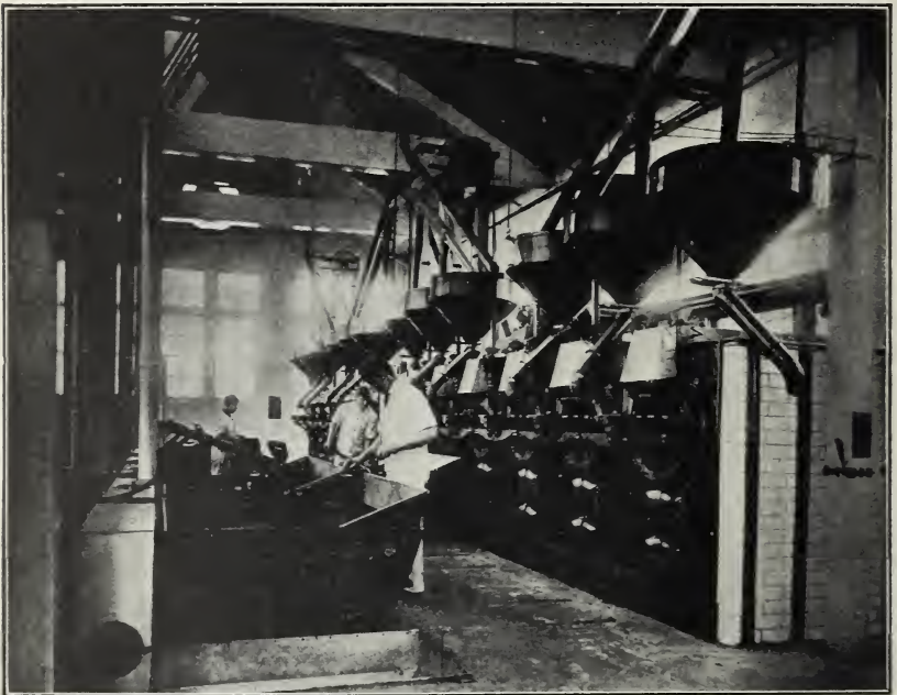
FIG. 1.—A roasting and cooling equipment in a model peanut-butter factory.
