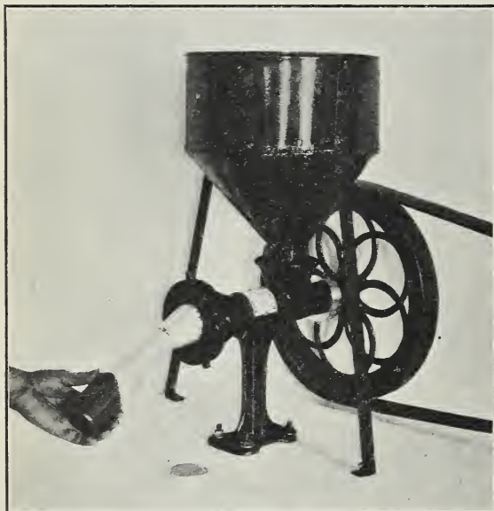
FIG. 6.—A small grinder commonly used in peanut-butter factories.
