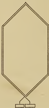
FIG. 76.—Two turn coil for a drum winding.
