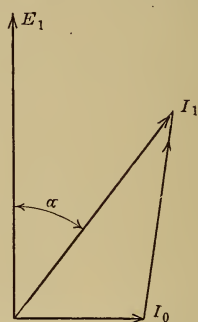
FIG. 345.—Ideal Full-load vector diagrams.
