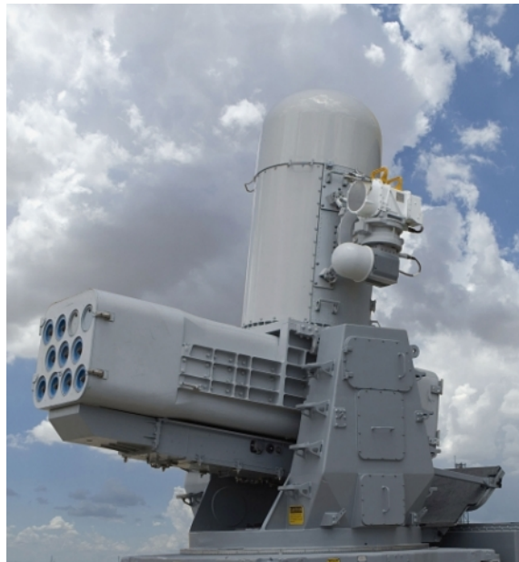
Figure 9. Mk 15 Mod 31 SeaRAM with Eleven-Cell RIM-116 Missile Launcher System. Source: Jane's IHS Markit (2017d).
