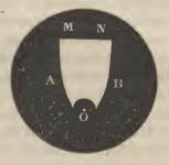
The dot (.) at O shows the position of the focus of a parabola, or one of the foci of a very long elipse. At or near this point the object to be viewed is to be placed. Concentric with this point the lower end of the glass paraboloid is removed by a hemispherical concavity to an extent sufficient to give working focal distance. A and B are sides of the paraboloid. M N is the upper limit of the glass, a
