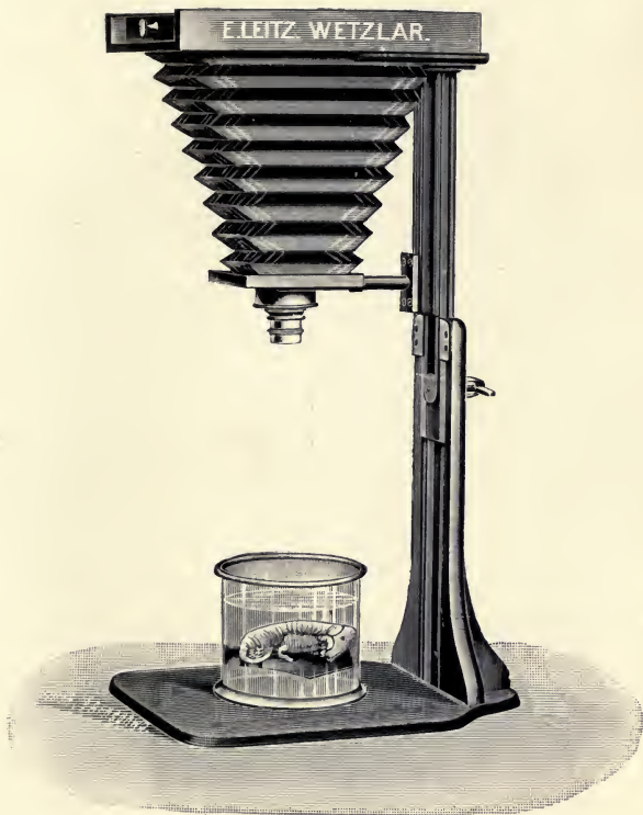
Fig. 138a.—Arrangement of camera with microsummar lens, when used for photographing opaque objects.
