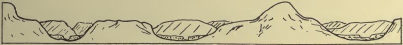
Fig. 28. Diagrammatic view of a region that has been reduced to base level and then rejuvenated; the rivers have cut valleys, forming isolated hills whose even tops indicate the former level of the land. The highest hills indicate prominences above the general level of the peneplain.
